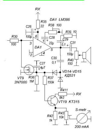
By resistor R42 we calibrate indications of S-meter, as which it is possible to apply the milliammeter with a current of arrow full deflexion up to 200-300mkA. At feeding of 50mkV on antenna input of the transceiver, the arrow of S-meter must show 9 points.
