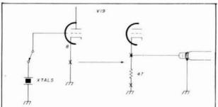
Heterodyne Oscillator: bandpass board, Tube V19, Pin 8 (cathode). This cathode is normally grounded. Break foil at X, solder 470 watt resistor across break. Connect center of coax to tube pin side, shield to adjacent foil ground. Coax goes to phono jack on rear of chassis.
