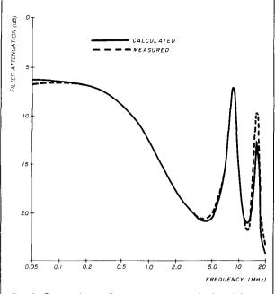
fig. 4. Comparison of measured and calculated filter response.
