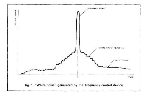
ent manufacture. I next cut out my external VFO (a PLL device) and cut in the internal VFO, which did not use PLL. I could thus test one frequency generation scheme against another at the push of a button. Using the internal VFO, the white noise disappeared immediately! My carrier was squeakyclean right up to my S9 plus 30-dB signal with no apparent sideband noise.
