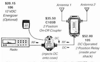
This system operates from 1.5 to 180 MHz and handles 1250 RF watts. Use our antenna switching kit and eliminate excess coax runs. With this kit and a single run of coax, you can switch between your antennas remotely. Use to add an antenna at modest cost, or change array direction.
