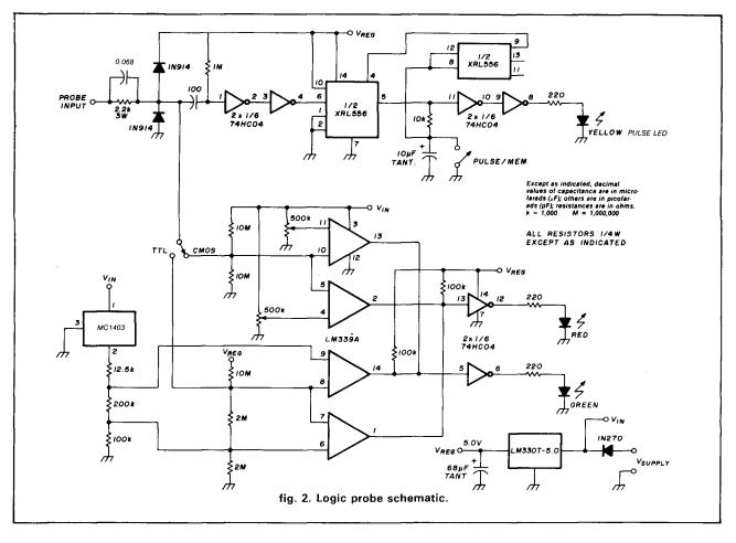
a wide range of supply voltages — 2 to 6 volts. This is useful because of the approximately 1-volt drop across the probe power supply. The 1-megohm resistor connected from the input to  $V_{REG}$  is a pullup resistor used to prevent the CMOS input from floating and erroneously triggering. The incoming pulses are put through two inverters which buffer the original pulse and square up the waveshape.
