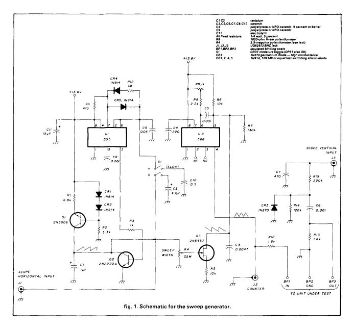
survived many hours of operation. R3, the 1-kilohm resistor in series with Q2 base, is near the maximum value that allows the collector to be driven close to ground.
