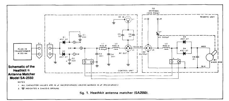
used to tune out the reactive inductance of one leg of the antenna as you move away from the design frequency. This allows the transmitter to see close to a 50-ohm impedance over a wider portion of the band. This "magic" is accomplished by varying the capacitor over its tuning range and adjusting for minimum SWR.
