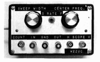
Photo 1. BP1 is labeled IN. Connect to input filter under test. BP3 is labeled OUT. Connect to output of filter under test. Positive going pulses about 5 microseconds long occur at the output, pin 3, at 40-millisecond intervals (fast rate) and at about 480-millisecond intervals (slow rate).
