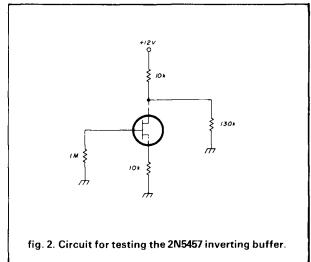
volts. The value of the 130-kilohm resistor can be varied  $\pm 20$  percent if necessary.
