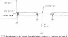
VFO: bandpass circuit board. Sampling coax connects to point on board where output coax of tube V20 connects. Connect coax center conductor to the foil point adjacent to high side of R221 (47 ohms).
