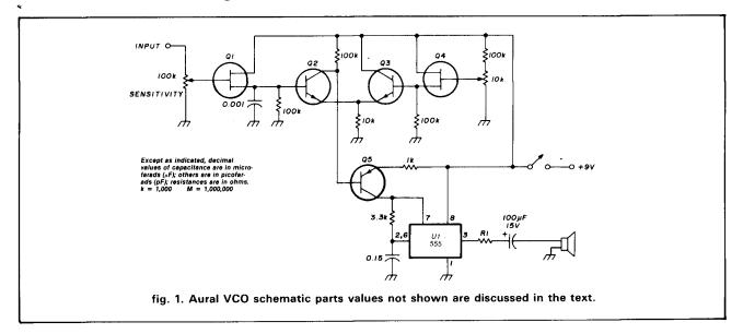
**Being an avid 2-meter foxhunter**, I'm always willing to try out any new gadget that might serve that end. This article describes a circuit, shared with me by Don Lèwis, KF6GQ, for an RF sniffer which produces a tone that rises in frequency as the signal gets stronger. Ideas for a number of useful Amateur applications will be discussed.
