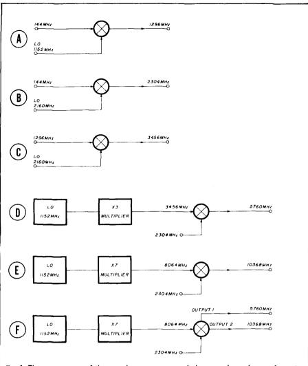
fig. 1. These are some of the popular or recommended conversion schemes for getting on the Amateur microwave bands. In all cases, the frequencies shown will place you near the most common operating frequencies listed in table 4. (See text for explanation of figs. 1A through 1F.)
