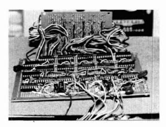
Photo D. A closer view of the bottom and digit boards illustrates interconnections.
