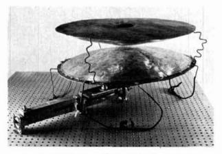
fig. 5B. Prototype X-band biconical horn.
