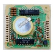
It is a well known fact that the RAM boards in some of the older ICOM radios have in them have volatile memory contents which need a lithium battery backup. The data in this RAM retains as long as the battery works fine. Usual life of this factory installed battery is between 7 to 15 years, depending on the working and storage conditions of the radio. There is no evident problem if the battery is replaced in time. You could replace the battery by using the procedure mentioned in this Icom URL:
