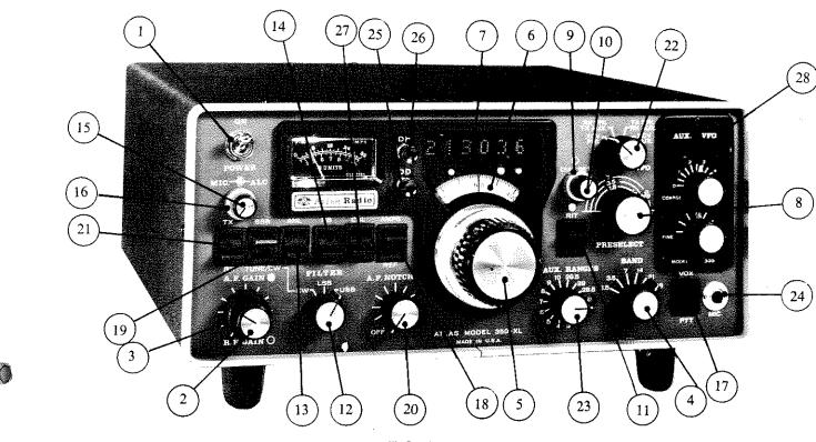
as cause splatter up and down the band. ALC will help reduce this danger, but it is still possible to overmodulate, so MIC Gain must be carefully adjusted.
