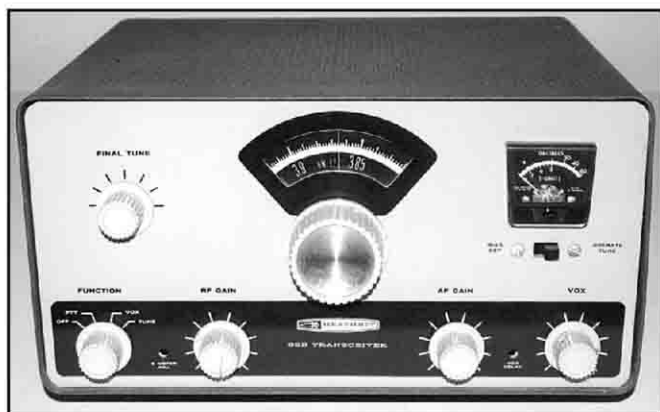
Figure 1—Heathkit HW-12 SSB transceiver, introduced and first sold in 1963.
