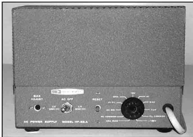
Figure 5—The Heathkit HP-23A power supply. Note the 11-pin socket that needed a plug and the 2 conductor ac cable that was replaced with a 3 conductor grounded type.
